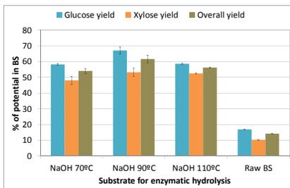
**Fig. 3a** – Glucose, xylose and overall (glucose + xylose) yields of NaOH extrudates submitted to enzymatic hydrolysis compared to hydrolysis of untreated BS. Yields are calculated as the amount of sugars produced by hydrolysis of the extrudate divided by the initial amount of glucose, xylose or glucose plus xylose in 100 kg of raw BS.
