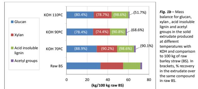
**Fig. 1b** – Mass balance for glucan, xylan, acid insoluble lignin and acetyl groups in the solid extrudate produced at different temperatures with KOH and comparison to 100 kg of raw barley straw (BS). In brackets, % recovery in the extrudate over the same compound in raw BS.
