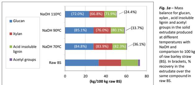
**Fig. 1a** – Mass balance for glucan, xylan, acid insoluble lignin and acetyl groups in the solid extrudate produced at different temperatures with NaOH and comparison to 100 kg of raw barley straw (BS). In brackets, % recovery in the extrudate over the same compound in raw BS.
