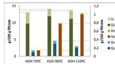
**Fig. 2b** – Composition of filtrate in g per 100 g of soluble solids (SS), insoluble solids (IS), monomeric glucose (Gm), oligomeric glucose (Go), monomeric xylose (Xm) and oligomeric xylose (Xo).
