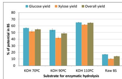
**Fig. 3b** – Glucose, xylose and overall yield of KOH extrudates submitted to enzymatic hydrolysis compared to hydrolysis of untreated BS. Yields are calculated as the amount of sugars produced by hydrolysis of the extrudate divided by the initial amount of glucose, xylose or glucose plus xylose in 100 kg of raw BS.
