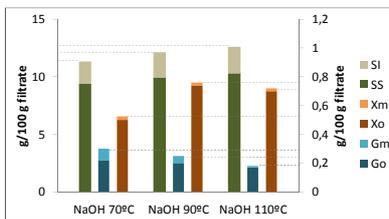
**Fig. 2a** – Composition of filtrate in g per 100 g of soluble solids (SS), insoluble solids (IS), monomeric glucose (Gm), oligomeric glucose (Go), monomeric xylose (Xm) and oligomeric xylose (Xo).
